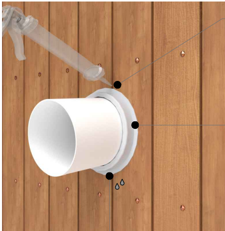
No sealant to drain
