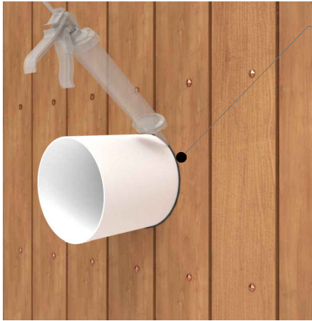
Continuous weather seal around pipe
